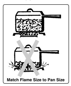
Match the flame to the bottom diameter of the pan. The flame should be the same size as the pan or slightly smaller. Small utensils and high flames result in energy loss and increase the potential for burns.
